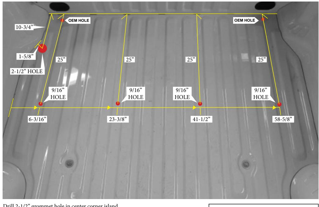
Drill 2-1/2" grommet hole in center corner island. Drill 9/16" holes in center between ribs Updated: 8-12-20
